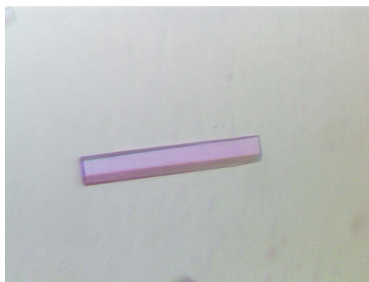
Figure 3 Thick hexagonal rod-shaped crystal. These crystals appeared using trisodium citrate as a precipitant in the presence of 10 mM trimethylamine–HCl. The crystals grew in a week to approximate dimensions of 0.5 × 0.1 × 0.1 mm.
