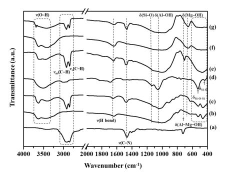
**Figure 2.** FT-IR spectra of (**a**) CTA, (**b**) unmodified Mt, (**c**) CTA-Mt, (**d**) unmodified mica, (**e**) CTA-Mica, (**f**) unmodified Ht, and (**g**) CTA-Ht.
