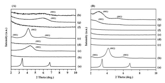
**Figure 3.** XRD patterns of: (**A**) (**a**) CTA, (**b**) pristine PP, (**c**) CTA-Mt, (**d**) 6 mass % CTA-Mt/PP nanocomposite, (**e**) CTA-Mica, (**f**) 6 mass % CTA-Mica/PP nanocomposite, (**g**) CTA-Ht, and (**h**) 6 mass % CTA-Ht/PP nanocomposite; (**B**) (**a**) CTA, (**b**) CTA-Mica, (**c**) pristine PP, (**d**) 1 mass % (depending on content of CTA-Mica/PP nanocomposite), (**e**) 3 mass %, (**f**) 6 mass %, (**g**) 9 mass %, and (**h**) 12 mass %.
