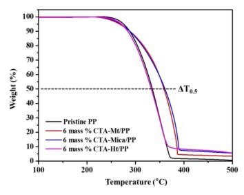
Figure 5. TGA curves for the 6 mass % CTA-clay nanocomposites.
