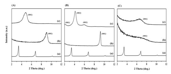
**Figure 1.** XRD patterns for (**A**) (**a**) CTA, (**b**) unmodified Mt, and (**c**) CTA-Mt; (**B**) (**a**) CTA, (**b**) unmodified mica, and (**c**) CTA-Mica; and (**C**) (**a**) CTA, (**b**) unmodified Ht, and (**c**) CTA-Ht.
