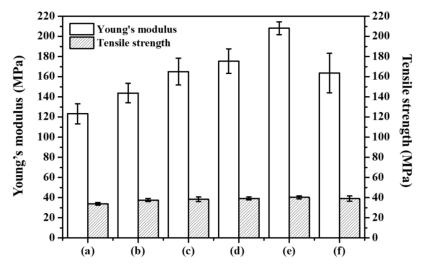
**Figure 7.** Mechanical properties analysis: Young's modulus and tensile strength of (**a**) pristine PP, (**b**) 1 mass % (depending on content of CTA-Mica/PP nanocomposite), (**c**) 3 mass %, (**d**) 6 mass %, (**e**) 9 mass %, and (**f**) 12 mass %.
