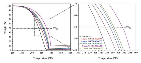
Figure 6. TGA curves for CTA-Mica/PP nanocomposites.
