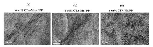
**Figure 4.** TEM images of (**a**) 6 mass % CTA-Mica/PP, (**b**) 6 mass % CTA-Mt/PP, and (**c**) 6 mass % CTA-Ht/PP nanocomposites.
