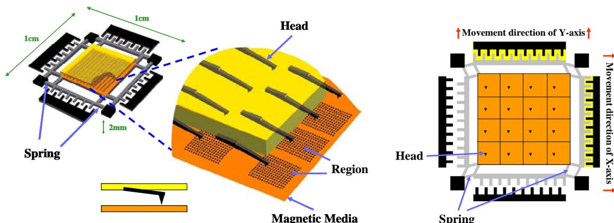
Fig. 1. Physical structure of a MEMS-based storage device [3]. There are thousands of regions on the magnetic media and a read/write head for each corresponding region. The magnetic media moves along two directional axes,  $x$  and  $y$ .
