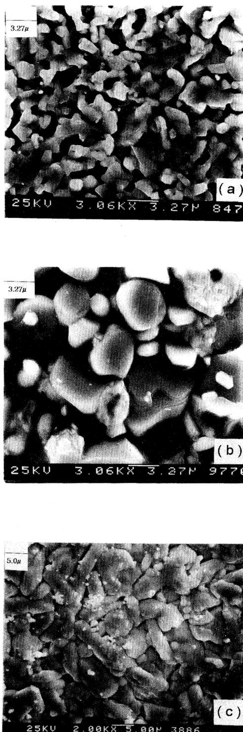
FIG. 1. (a) An SEM picture of sample *A1* (bulk *A*). Most grains are about 1–2 μm in size. (b) An SEM picture of sample *B* (bulk *B*). Most grains appear 3–6 μm in size, larger than the average grain size in sample *A1* (bulk *A*). (c) An SEM picture of sample *C* (bulk *C*). Most grains appear 3–6 μm in size, comparable to the grain size in sample *B* (bulk *B*) and larger than the average grain size in sample *A1* (bulk *A*).
