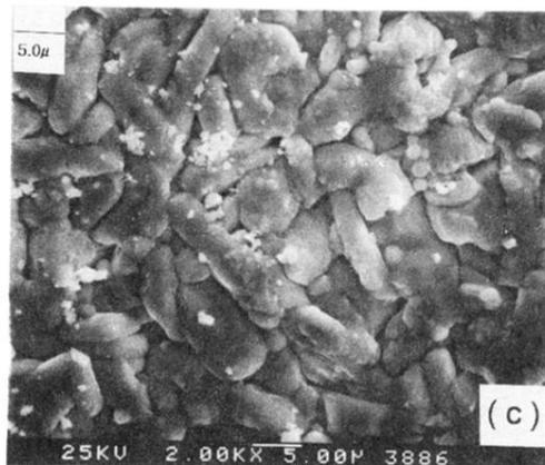
FIG. 1. (a) An SEM picture of sample *A1* (bulk *A*). Most grains are about  $1\text{--}2\ \mu\text{m}$  in size. (b) An SEM picture of sample *B* (bulk *B*). Most grains appear  $3\text{--}6\ \mu\text{m}$  in size, larger than the average grain size in sample *A1* (bulk *A*). (c) An SEM picture of sample *C* (bulk *C*). Most grains appear  $3\text{--}6\ \mu\text{m}$  in size, comparable to the grain size in sample *B* (bulk *B*) and larger than the average grain size in sample *A1* (bulk *A*).
